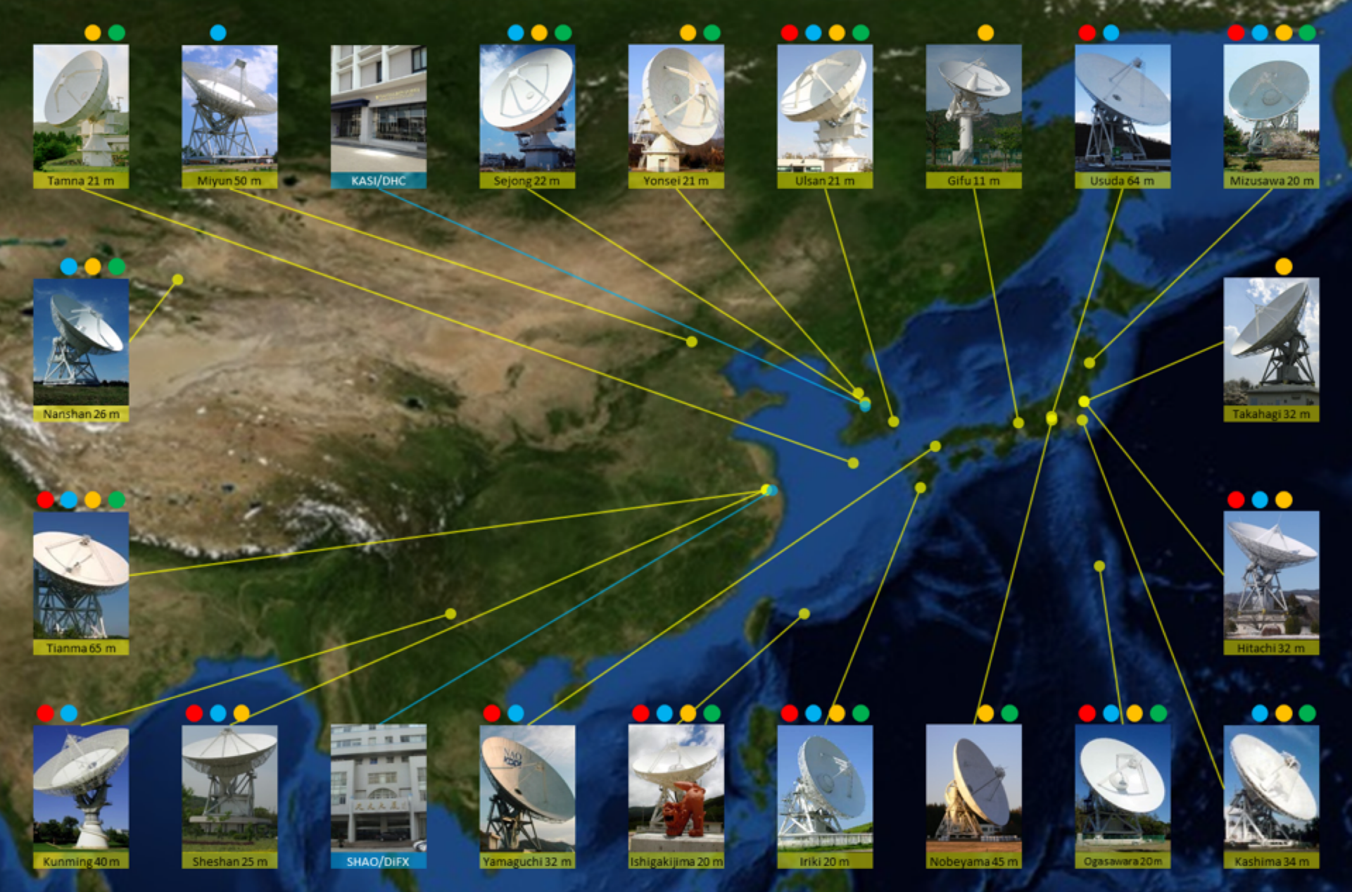
The East Asian VLBI Network (Image Credit: Reto Stöckli, NASA Earth Observatory) ● 6.7 GHz ● 8 GHz ● 22 GHz ● 43 GHz
