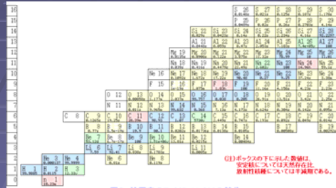
図3 核図表のZ<17, N<14の部分 [出典] JAERI Nuclear Data Center: WWW Chart of the Nuclides 2003. http://wwwnds.tokai.jaeri.go.jp/CHN0/index.html
